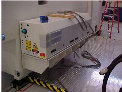
A coaxial laser mounting (Photo with permission of TRUMPF Inc.)
