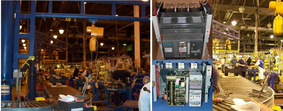
Large Frame Breakers production lines (Photo with permission of General Electric)
