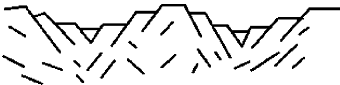
Figure 3. Horst and graben structures; the downthrown and upthrown blocks form the grabens and horsts, respectively.
