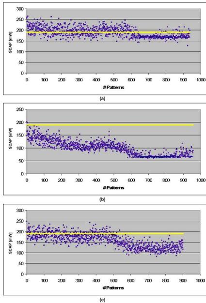
Fig. 9. Switching cycle average power (SCAP) in VDD network for the low switching activity test patterns generated in three cases: (a) *fill-1*, (b) *fill-0* and (c) *fill-adjacent*
