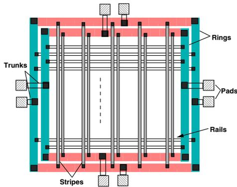
Fig. 1. Power/Ground Distribution Network.
