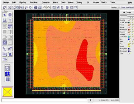
Fig. 4. IR-drop plot in VSS net for pattern  $P1$ .
