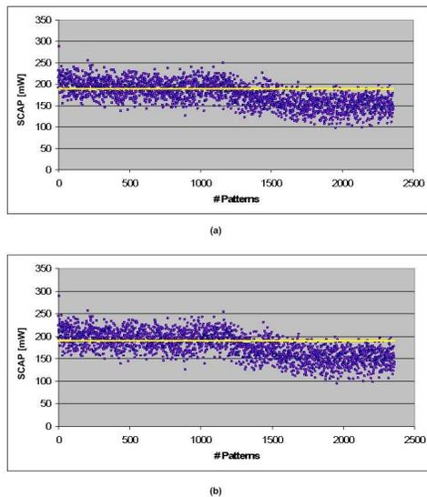
Fig. 7. Switching cycle average power (SCAP) measured for each transition fault test pattern (a) VDD network and (b) VSS network.
