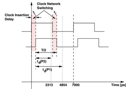
Fig. 2. Clock timing waveform used for dynamic IR-drop analysis.
