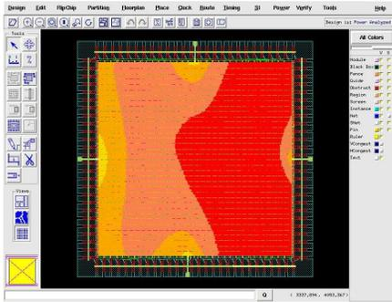
Fig. 5. IR-drop plot in VSS net for pattern  $P2$ .
