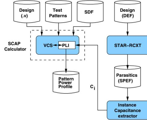
Fig. 6. SCAP calculator using Synopsys VCS simulator.
