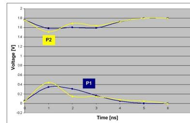
Fig. 3. IR-drop effects on VDD and VSS during pattern *P1* and *P2* application within 7 ns capture window.
