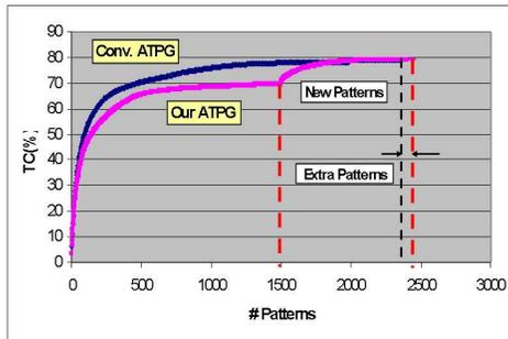
Fig. 10. Test coverage curves for conventional ATPG and our new supply aware ATPG.
