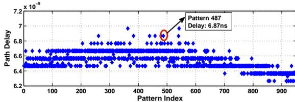
Figure 3: Path delay based on fast-SPICE simulation for 950 random-filled patterns.
