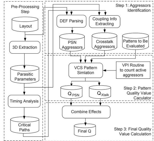
**Figure 2: Flow diagram of the pattern quality value calculation procedure.**
