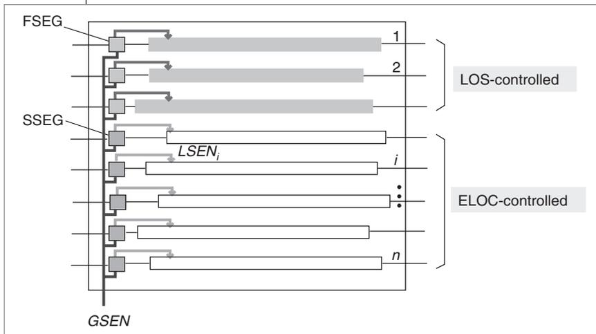
**Figure 6. Hybrid scan test architecture: FSEG cells driving LOS-controlled scan chains, and SSEG cells driving ELOC-controlled scan chains.**
