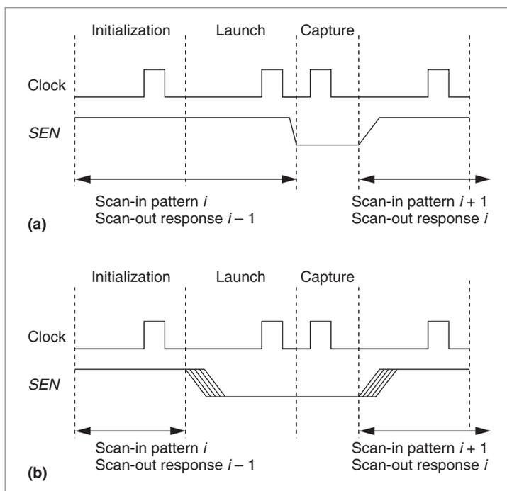
**Figure 1. Transition delay fault pattern generation methods: launch-off-shift (LOS) (a) and launch-off-capture (LOC) (b).**
