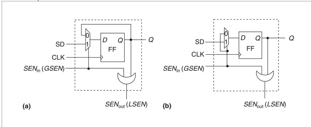
**Figure 3. LSEG cells: slow scan-enable generator (SSEG) cell (a) and fast scan-enable generator (FSEG) cell (b).**
