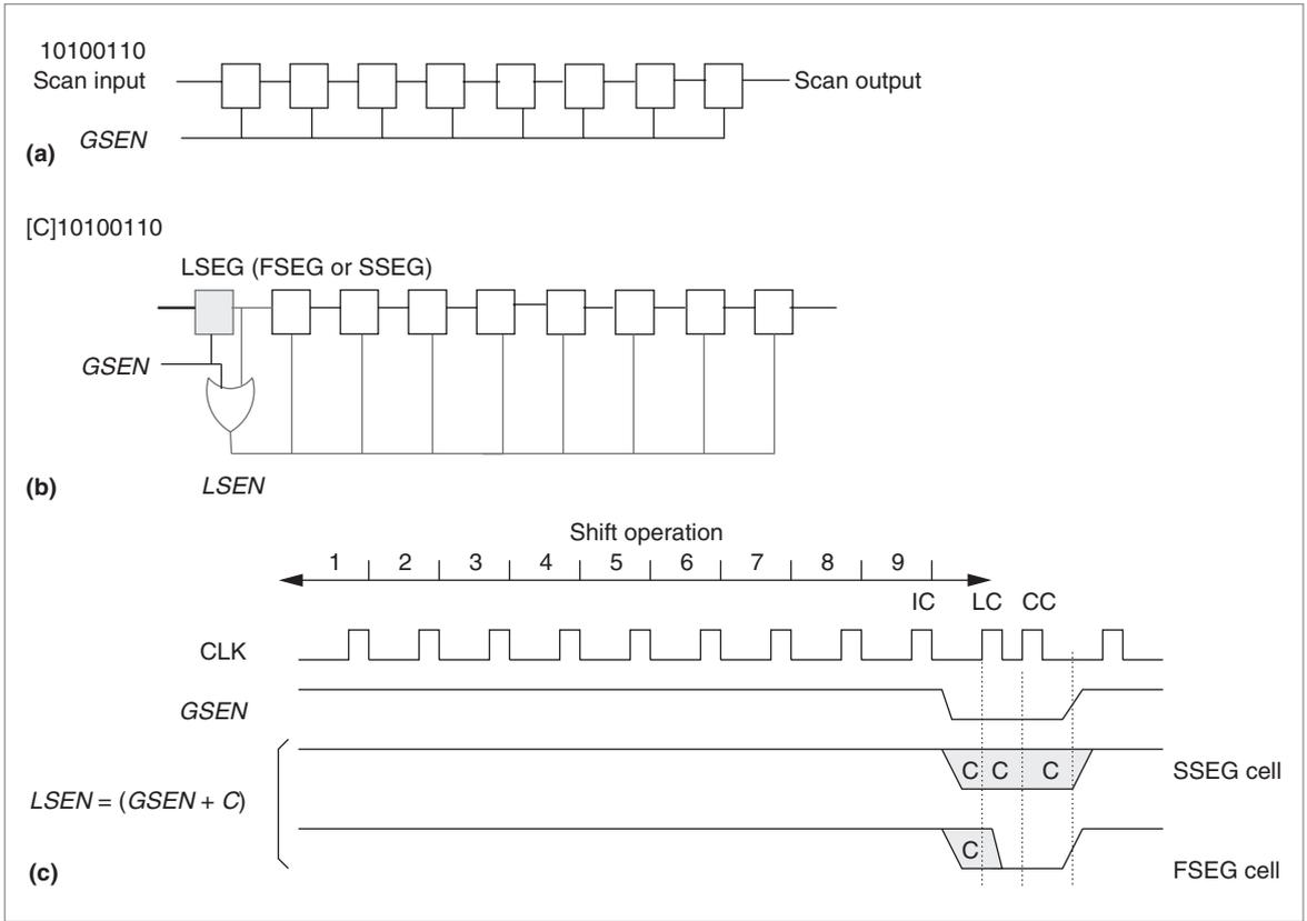
**Figure 4. LSEG cell operation: Scan chain architecture (a), LSEN generation using LSEG (b), and LSEN generation process and waveforms (c).**
