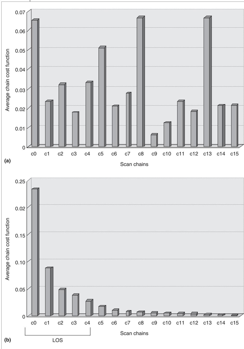
**Figure 8. Average cost function before (a) and after (b) scan insertion based on controllability and observability.**
