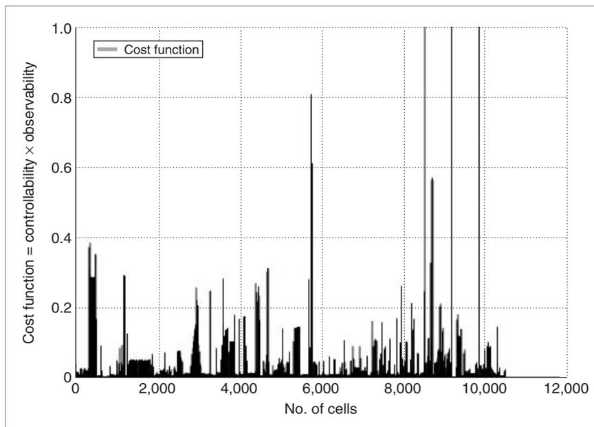
**Figure 7. Cost functions of scan flip-flops in case study design.**
