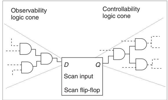
**Figure 5. Scan flip-flop controllability-and-observability measure.**
