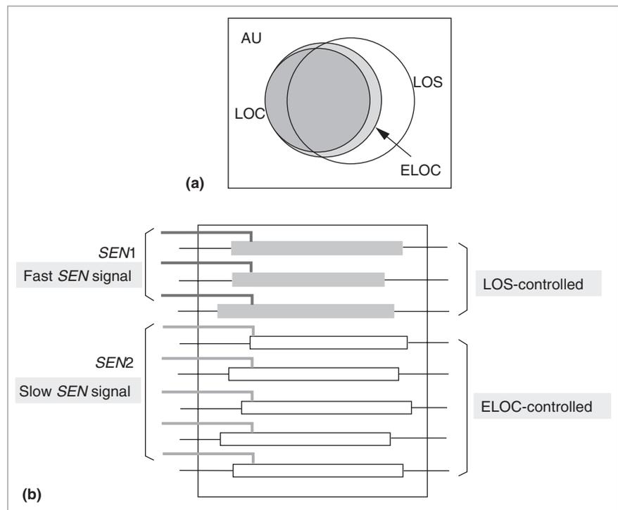
**Figure 2. Hybrid method analysis and architecture: Fault analysis of LOS, LOC, and ELOC techniques (a), and hybrid scan architecture: with LOS-controlled scan chains using fast *SEN* signal and ELOC-controlled scan chains using slow *SEN* signal (b).**
