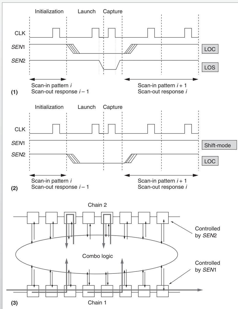
**Figure A. Previously proposed techniques: *SEN* waveforms in hybrid scan technique (1), *SEN* waveforms in enhanced LOC (ELOC) technique (2); ELOC controllability—chain 1 used in shift mode, and chain 2 in functional mode (3).**
