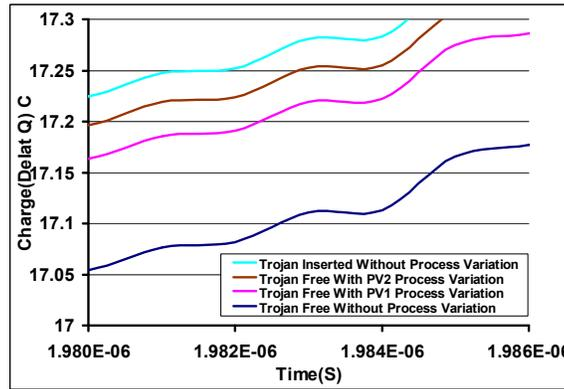
**Figure 6** Charge measurement for s38417 with 20-input Comparator (here, PV2 represents the worst-case variations and PV1 represents lower variations)
