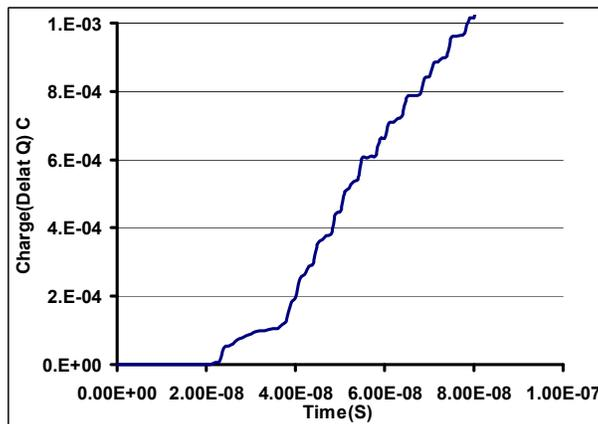
**Figure 7.** Charge measurement for s38417 with 5-input Comparator with no process variations
