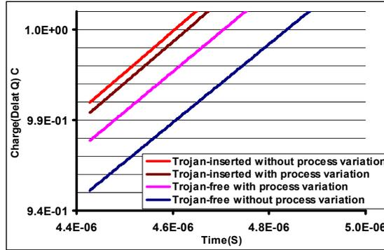
**Figure 5.** Charge measurement for s38417 with 3-bit Counter considering the worst-cased process variations for Trojan-free circuit
