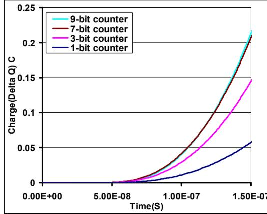
**Figure 4.** Charge measurement for s38417 with four Counter Trojans inserted into s38417
