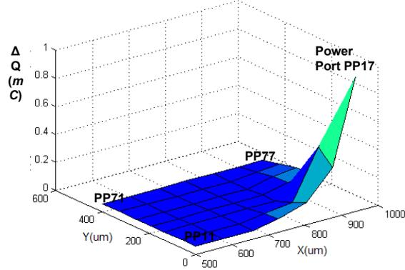
**Figure 3.** Current difference measured on power port 17
