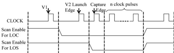
Figure 2: Using multiple capture cycles
