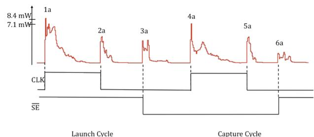
Figure 5: Transient analysis during LOS for b05
