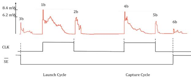
**Figure 6: Transient analysis during LOC for b05**
