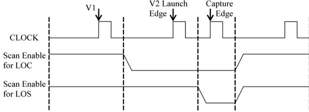
Figure 1: Waveforms of LOC and LOS
