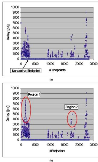
**Figure 7: Path delay variation of a test pattern in two cases: (a) no IR-drop effects and (b) scaled cell delays due to IR-drop effects.**
