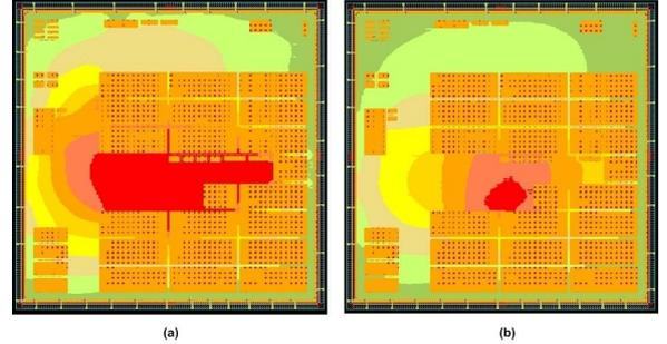
**Figure 3: VDD IR-drop plots using SCAP model for two patterns (a) P1 and (b) P2.**
