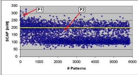
**Figure 2: SCAP measured in block B5 for transition fault pattern set in *clkA* domain.**
