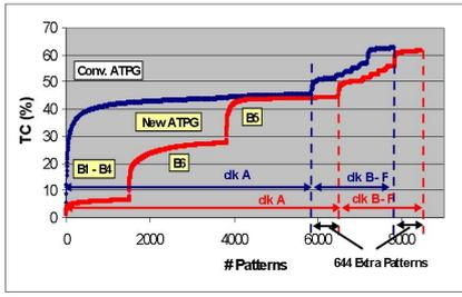
Figure 4: Test coverage curves for conventional ATPG and the new pattern generation procedure.
