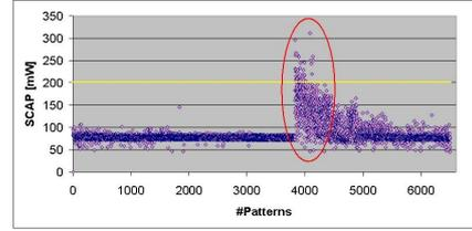
Figure 6: Switching cycle average power (SCAP) measured on VDD network for each pattern in the new test pattern set (*clkA* domain pattern set).
