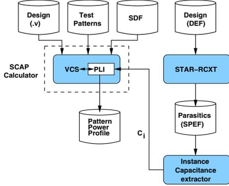
Figure 5: SCAP calculator using Synopsys VCS simulator.
