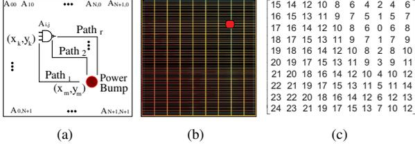
Figure 3. Resistance path and resistance network: (a) Resistance paths from an instance or region to a power bump; (b) least resistance plot from SOC Encounter for a specific power bump; (c) least resistance network.
