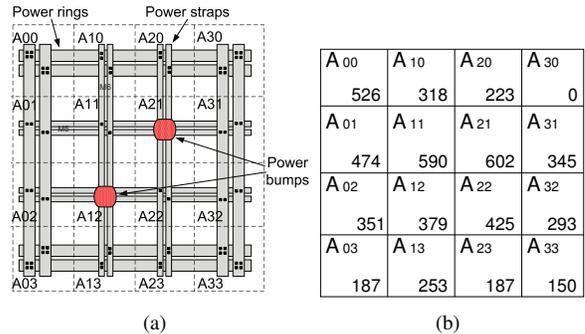
Figure 2. Layout partitions: (a) An example of the power straps being used to partition the layout into regions. (b) An example of  $WSA_A$  matrix.
