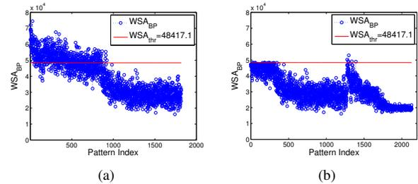
Figure 5. WSA plot for b19 benchmark: (a) original pattern set; (b) final low-power pattern set
