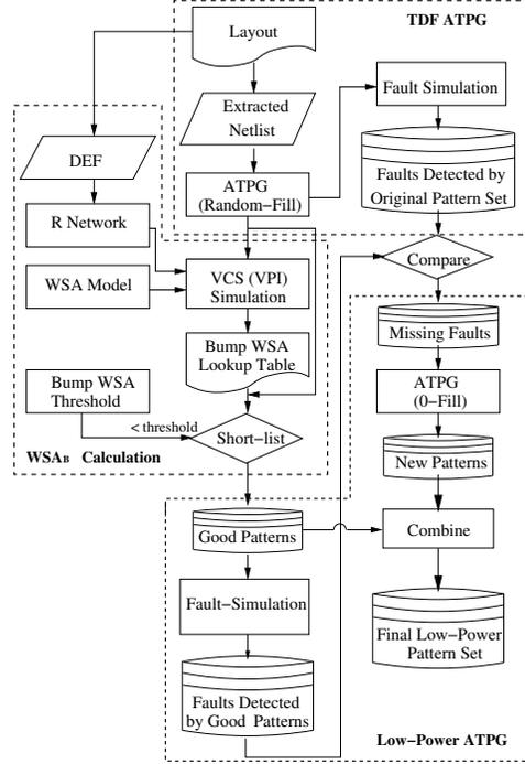
Figure 4. Flow diagram of pattern grading and power-safe pattern generation.
