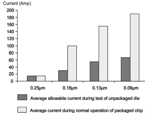
Figure 1. Power availability during wafer testing [12].
