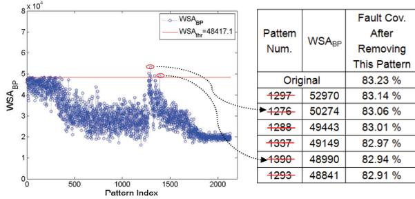
Figure 6. Fault coverage loss analysis for b19 benchmark when removing the remaining high-power patterns from the pattern set.
