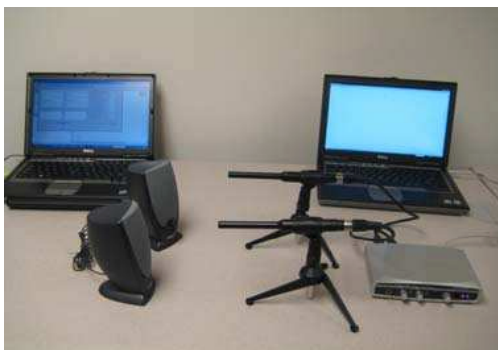
Fig. 4. The MIMO-OFDM prototypes (left) PC based and (right) DSP based implementation
