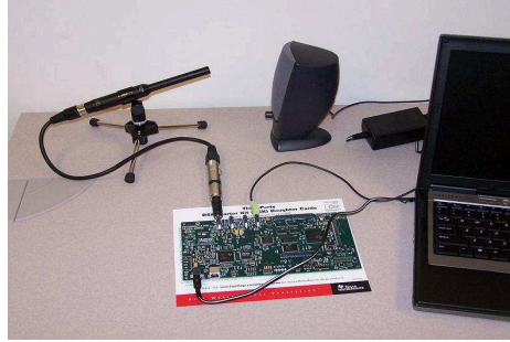
Fig. 2. The DSP-based prototype for real-time one-way communication
