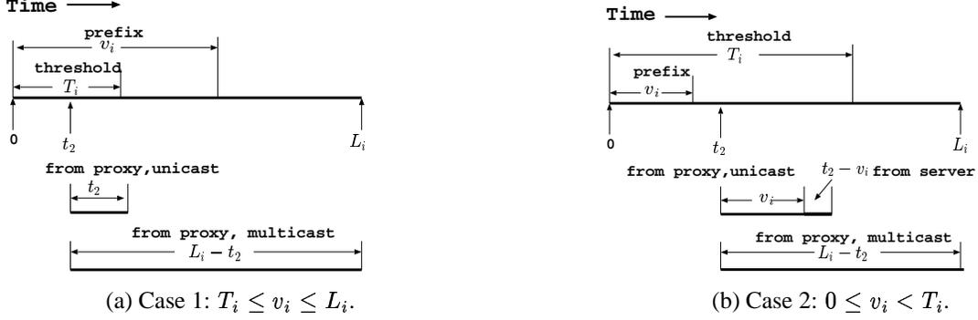
Fig. 3. Multicast patching with prefix caching (MPatch).
