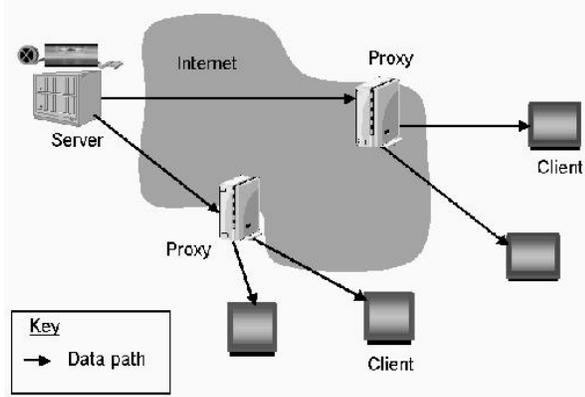
Fig. 1. **Streaming video in the Internet:** The video stream originates from a remote server and travels through the network to the end client. The proxies performing prefix caching are located close to the clients, e.g., at the head-end of the local access network.
