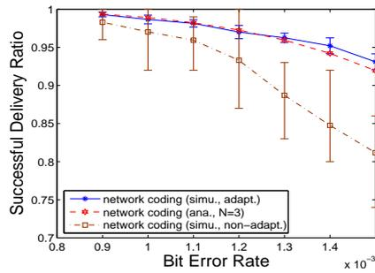
Fig. 5. Transmission-range adaption in uniform random deployment.
