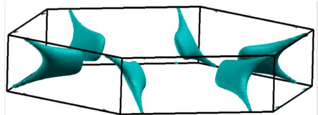
A quasi-1D feature predicted to occur in the valence band of  $\text{AgBiSe}_2$ . Analysis indicates the feature may substantially enhance thermoelectric performance [3].
